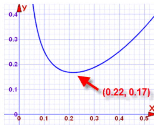
Plot of y = 0.3(0.08/x + 4x^2) x is width, and y is cost
